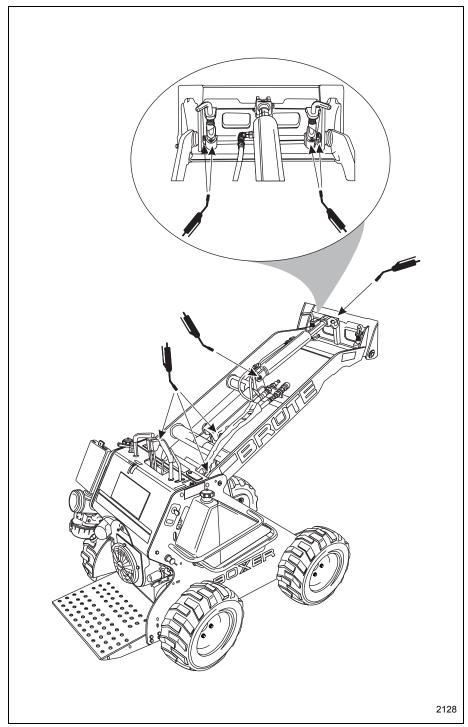
Figure 3–4 Lubrication Points
